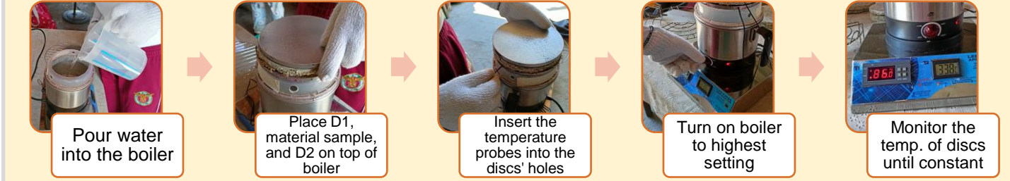
Figure 7. Identification of Steady State Temperatures
