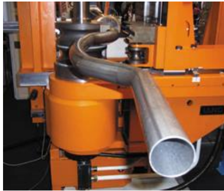
Figure 21. Tube Bending
