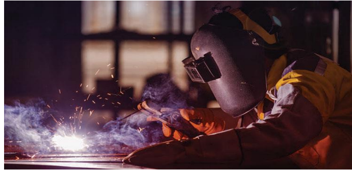
Figure 24. Shielded Metal Arc Welding
