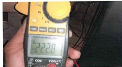
Voltage reading on the refrigerator outlet
